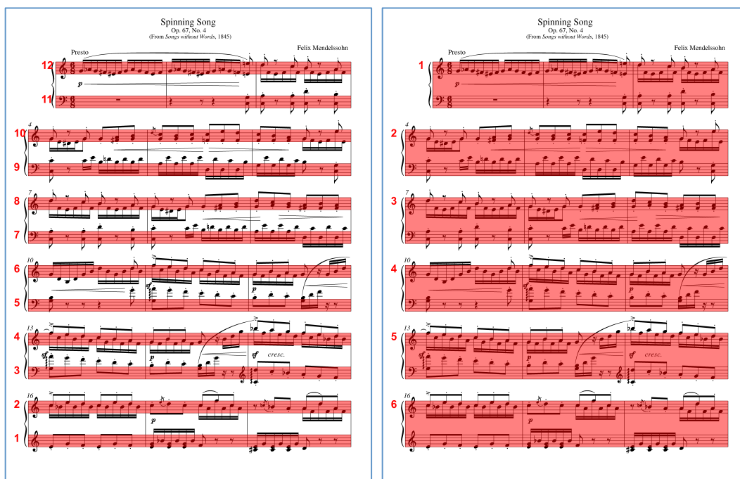
Figure 14: Staff highlighting in actual music using the hilitestaff program. The image on the left was processed with the command “ hilitestaff -n spin1.vec spin1.tif spinout.tif ”. The image on the left was created with the command “ hilitestaff -n -s2 spin1.vec spin1.tif spine2out.tif ” which highlights pairs of staves when adding the -s 2 option. Note that when highlighting multiple staves per system, the -n option will number from the top of the page down. See Appendix V starting on page 88 for the PMX data of this music.
